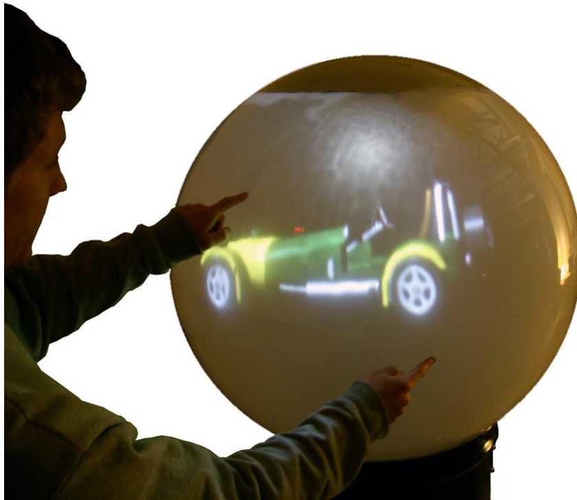
Figure 4.2. Scaling gesture. To scale a model, a user raises both hands. As the distance between the hands increases, the models is enlarged, as the distance decreases, the model is shrunk.
