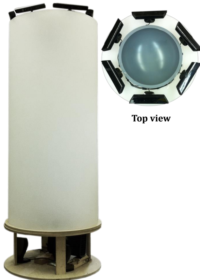
Figure 3.3. TeleHuman hardware: a cylindrical display surface with 6 Kinects and a 3D projector inside its base.
