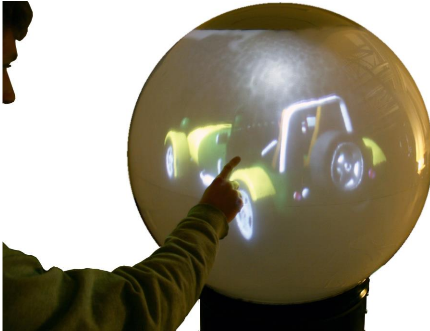
Figure 4.1. Rotation gesture. To rotate a model, a user raises a hand and then moves the hand horizontally or vertically. The axis of rotation is determined by whether the user moves their hand horizontally or vertically. This analogous to spinning the entire volume.
