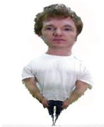
Figure 3.5. Textured 3D model with hemispherical distortion. When reflected off the convex mirror onto the cylinder, this produces a 3D model with proper proportions.
