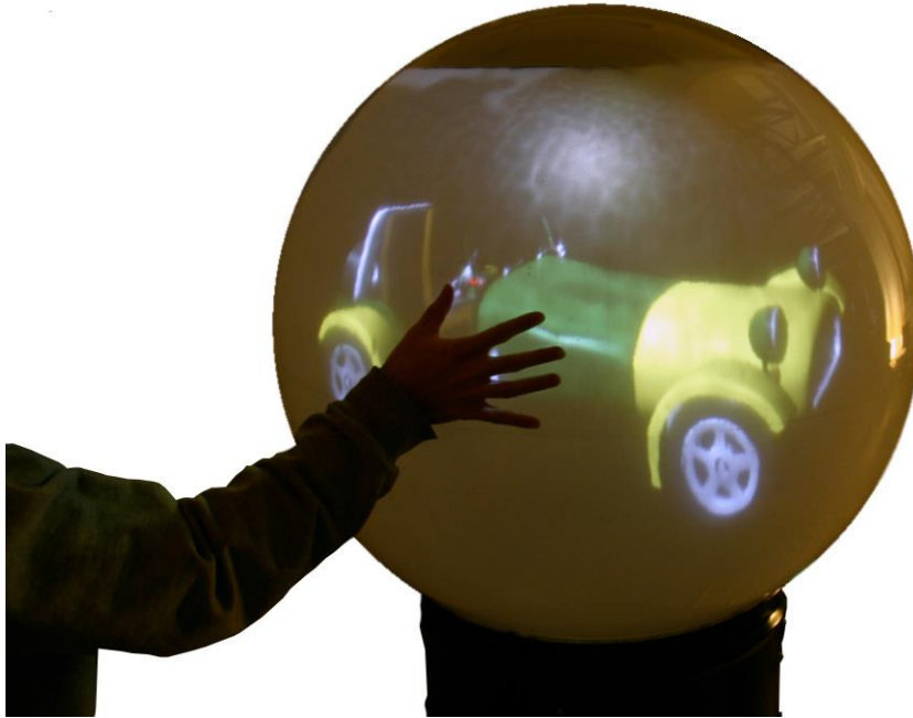
Figure 4.3. Model switching gesture. To change models, the user preforms a waving gesture. This is designed to represent the act of scrubbing the model off the display.
