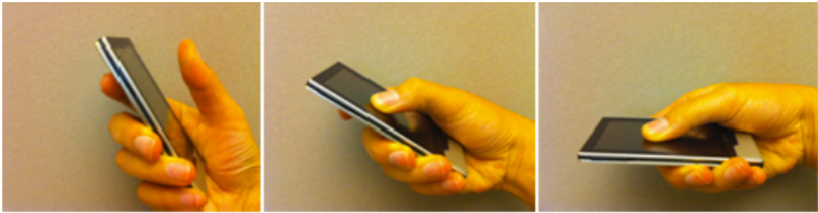
Figure 6. Augmenting touch input with tilt sensing. No zooming takes place until the thumb is placed on the screen (middle). Zooming is then mapped to the change in pitch (right).
