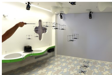
Figure 3. Creating a catenary archway with GridDrones by raycast selecting a backbone, then lifting. Secondary drones follow the actions.
