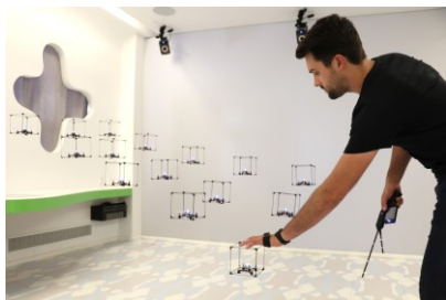
Figure 1. GridDrones system with an array of self-levitating physical voxels represented by small quadcopters.
