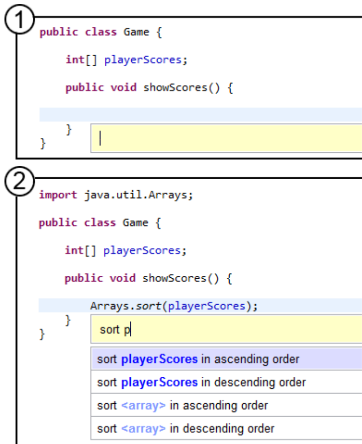
Figure 7. The SnipMatch plug-in for the Eclipse development environment. A keyboard shortcut opens the search window (1) at the programmer’s cursor position. Search results (2) are updated as the query is typed. The search query also affects integration: the local variable playerScores is included in the snippet (2). Snippet integration is previewed within the existing code.
