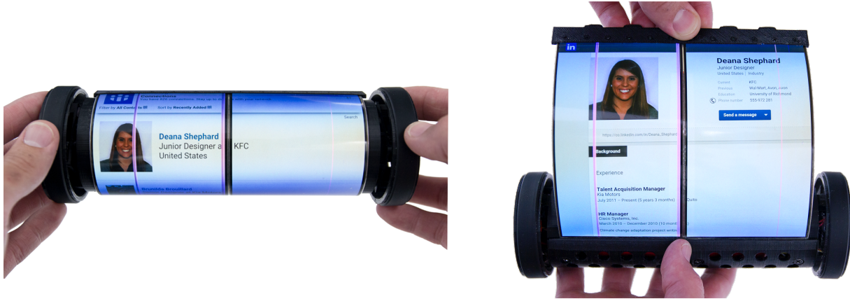
Figure 6: LinkedIn Rolodex app running on MagicScroll. Left: MagicScroll rolled showing the profile photo and summary. Right: MagicScroll expanded displaying the full LinkedIn information.
