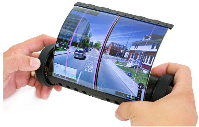
Figure 1. Unfolded MagicScroll prototype showing Street View navigation.
