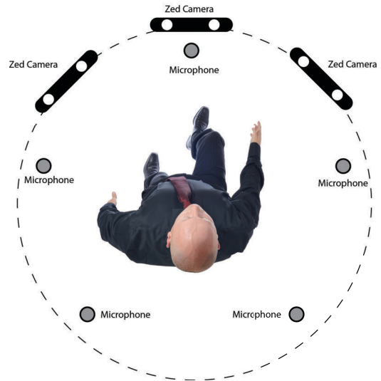
Figure 4. Diagram of remote capture system. Coverage is increased by adding 1 ZED camera every 20 degrees.
