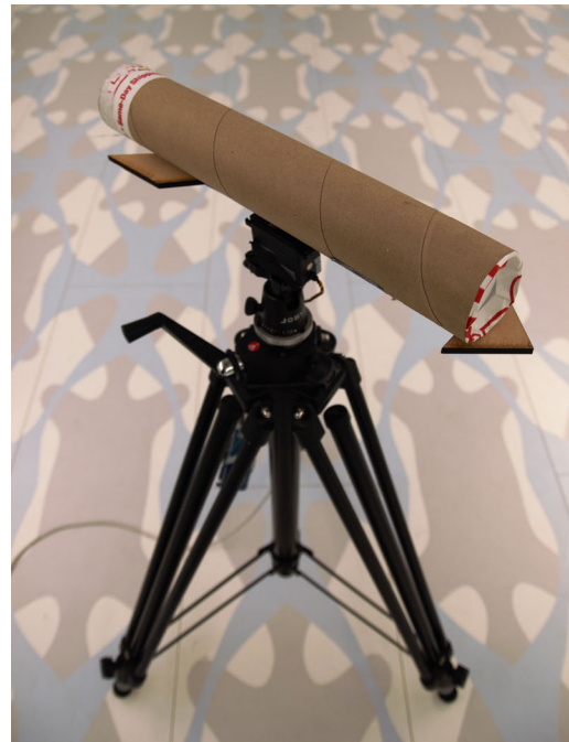
Figure 6. Physical tripod with cylindrical arrow and servo.
