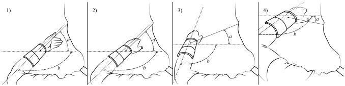
Figure 4. The kinematic model provides DisplaySkin with the angle between a user's eye and the device (a). DisplaySkin uses this angle to present information on visible area of the display. The model also provides the orientation of the device relative to a user's body (b), which is used to align the content horizontally (similar to Wilfinger et al. [41]).
