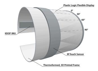
Figure 5. DisplaySkin hardware schematic.
