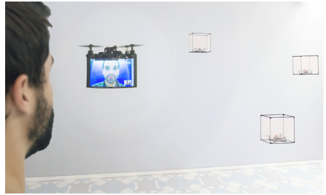
Figure 9. User inspecting a remote facility using a DisplayDrone with telepresence functionality.
